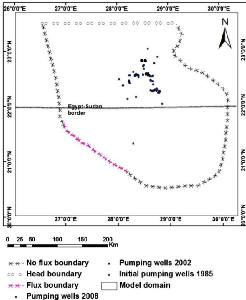
Fig. 3. The boundary conditions of the model area.
